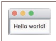
Figure 8-3 Displaying a label with text in a window
